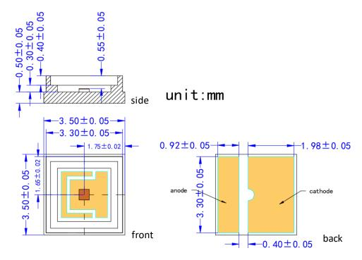
VD-0940C-020M-3A-2A0 with Substrate 3=CuAg and Package A=2016 (unit: mm)
