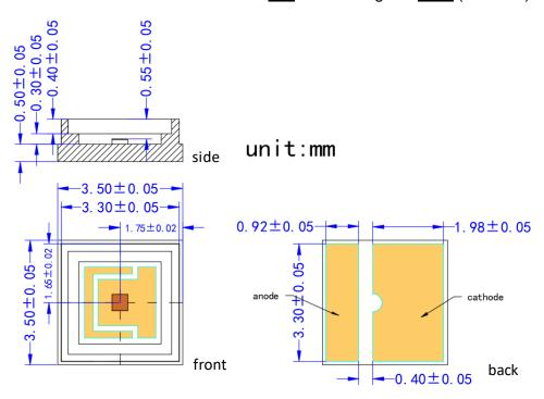
VD-0940I-004W-1D-2A0 with Substrate 1=AIN and Package D=5050 (unit: mm)
