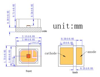
VD-0940I-200M-1C-2A0 with Substrate 1=AIN and Package C=3535 (unit: mm)
