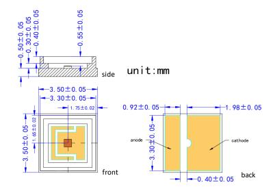
VD-0940I-200M-3A-2A0 with Substrate 3=CuAg and Package A=2016 (unit: mm)
